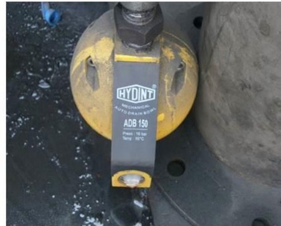
Automatic Drain Valve (mechanical type)
